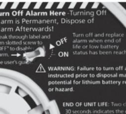
Turn the screw to the “OFF” location. This will deactivate the alarm, stop the low battery “chirp” and render the alarm safe for disposal by draining the battery.
