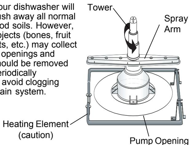
1. Remove tower base by turning counterclockwise.
